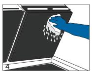
Rinse the upper and lower release sheets with a separate sanitizer-soaked grill cloth. Wipe until the grill cleaner residue has been fully removed.
