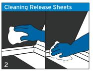
Wipe the upper and lower grill, prior to removing any release sheets, with a clean sanitizer-soaked grill cloth.
